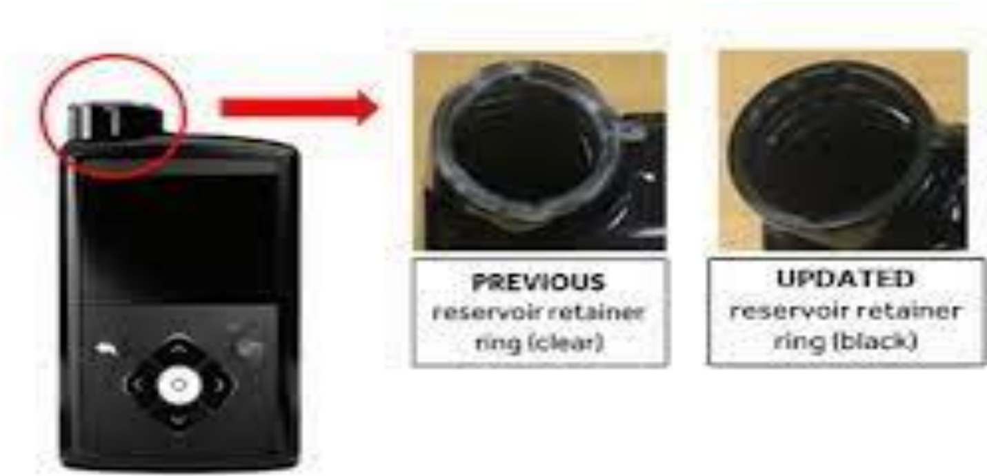
Image: Location of the retainer ring on the MiniMed™ 600 series insulin pump
