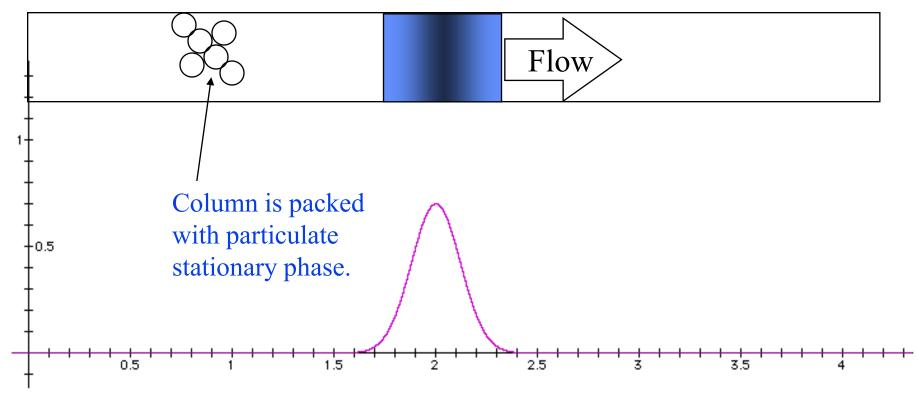
As a material travels through the column, it assumes a Gaussian concentration profile as it distributes between the stationary packing phase and the flowing mobile gas or liquid carrier phase.
