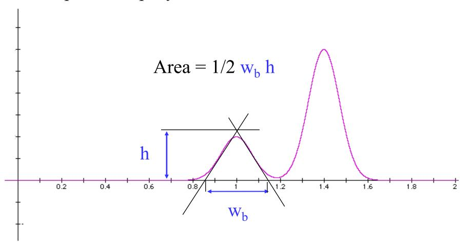
NOTE: the height is measured to the top of the tangents, which is above the actual curve peak.
