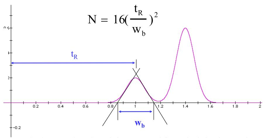
t<sub>R</sub> is the retention time; it is measured from the injection peak (or zero) to the intersection of the tangents.
