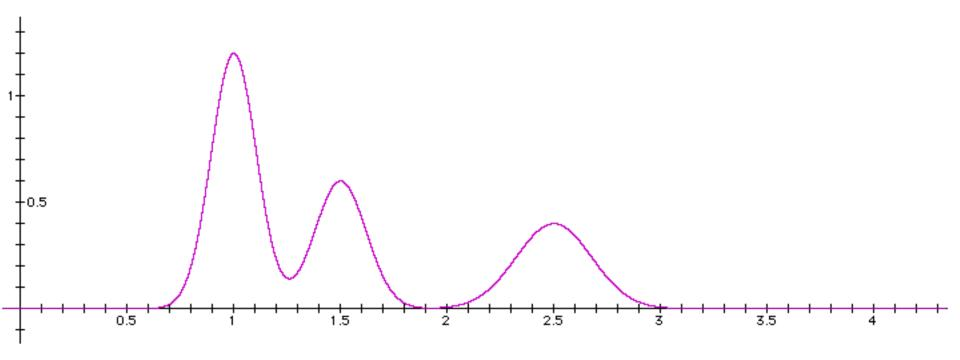
Note: The first two components were not completely separated. Peaks in general tend to become shorter and wider with time.
