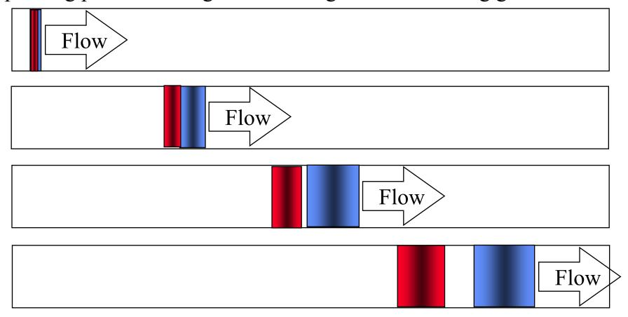
More volatile materials are carried through the column more rapidly than less volatile materials, which results in a separation.
