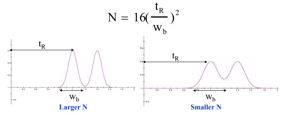
When the retention time,  $t_R$ , is held constant, the column that produces peaks with narrower bases,  $w_b$ , will be more efficient – have a greater N value.
