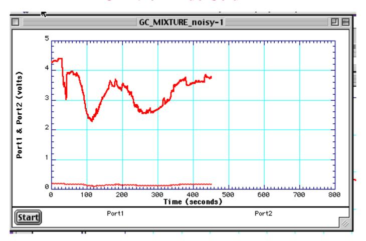
Poor: peaks are noisy, due to flickering flame, and elute slowly.To fix: Adjust sensor so that it is looking at the blue portion of the flame. (Verify the flame is blue.)
