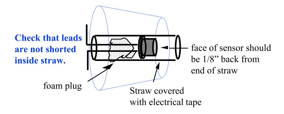
Note: The sensor should be tested by connecting to computer and checking voltage in light and with sensor face covered with your finger.
