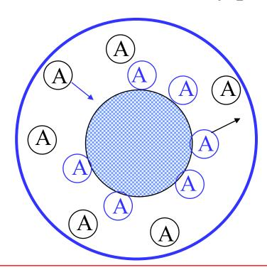
Cross Section of Equilibrium in a column. "A" are adsorbed to the stationary phase. "A" are traveling in the mobile phase. **K** = distribution coefficient *or* partition ratio
