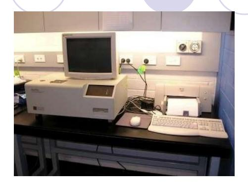
Photocorrelation Spectroscopy - **Brookhaven Zeta Plus** dilute msuspensions <5microns light scattering technique
