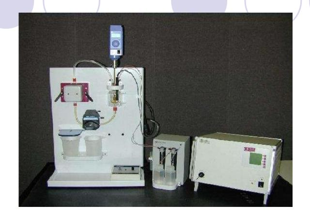
Electroacoustic - Colloidal Dynamics Acoustosizer powders/slurries < 10nm - up to 50 weight%
