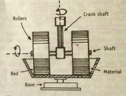
Figure 6-11. Construction of edge runner mill.
