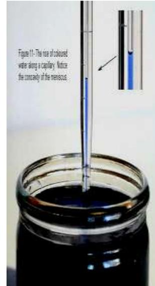
➤ If a capillary tube of inside radius =  $r$  immersed in a liquid that wet its surface, the liquid continues to rise in the tube due to the surface tension, until the upward movement is just balanced by the downward force of gravity due to the weight of the liquid
