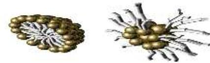
➤ **Inverted spherical micelles**
