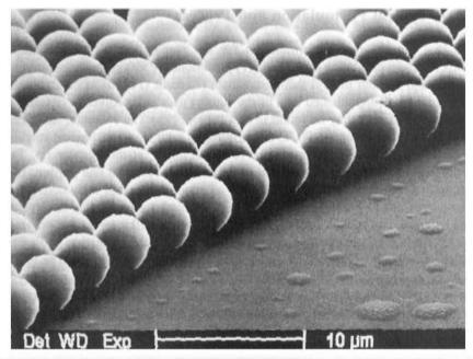
Figure 22.1 Scanning electron micrograph of polystyrene microspheres prepared by dispersion polymerization. (Photomicrograph courtesy of T. Groves/A. Rowley, liford Ltd)
