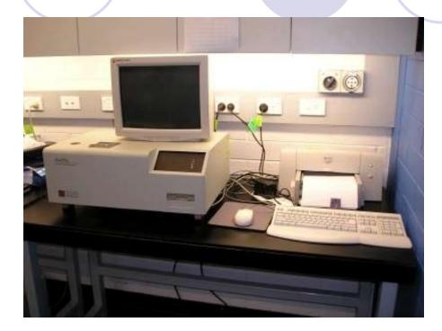
Photocorrelation Spectroscopy - **Brookhaven Zeta Plus** dilute msuspensions <5microns light scattering technique
