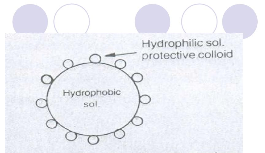
Fig. 5.8. Principle of protection by a protective colloid.
