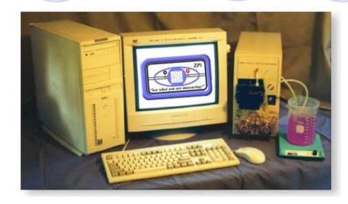
Electrophoresis - Zeta Mark 21 particles ~ .10 microns- 300 µm
