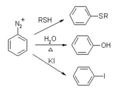
The Sandmeyer Reaction is a very important transformation in aromatic chemistry, because it can result in some substitution patterns that are not achievable by direct substitution.
