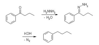
The reduction of aldehydes and ketones to alkanes. Condensation of the carbonyl compound with hydrazine forms the hydrazone, and treatment with base induces the reduction of the carbon coupled with oxidation of the hydrazine to gaseous nitrogen, to yield the corresponding alkane.
