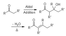
In some cases, the adducts obtained from the Aldol Addition can easily be converted (in situ) to  $\alpha,\beta$ -unsaturated carbonyl compounds, either thermally or under acidic or basic catalysis. The formation of the conjugated system is the driving force for this spontaneous dehydration. Under a variety of protocols, the condensation product can be obtained directly without isolation of the aldol.
