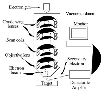
Fig. 11 Scanning Electron Microscope
