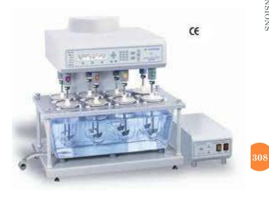
The apparatus consists of a cylindrical 1000- ml round bottom flask in a multiple – spindle dissolution drive apparatus and immersed in a controlled temp bath maintained
