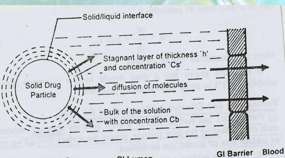
Dissolving Solid Drug GI Lumen GI Barn Fig. 2.11 Diffusion layer model for drug dissolution
