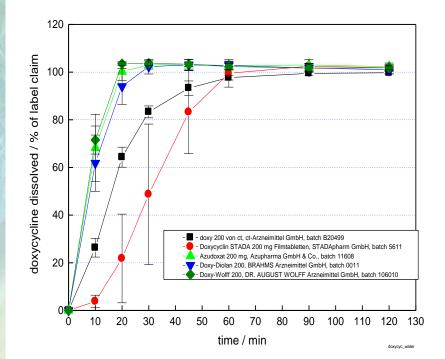
120 doxycycline dissolved / % of label claim 100 80 60 40 - X – doxy 200 von ct, ct-Arzneimittel GmbH, batch B20499 Doxycyclin STADA 200 mg Filmtabletten, STADApharm GmbH, batch 5611 20 Azudoxat 200 mg, Azupharma GmbH & Co., batch 11608 Doxy-Diolan 200, BRAHMS Arzneimittel, batch 0011 Doxy-Wolff 200, DR. AUGUST WOLFF Arzneimittel, batch 106010 ñ 10 20 30 40 50 60 70 80 90 100 time / min
