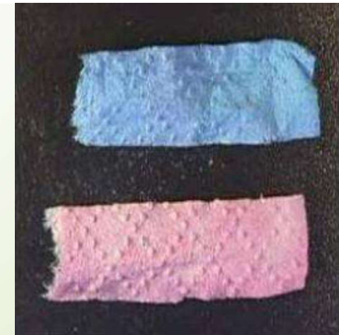
Blue cobalt-chloride paper turning pink in the presence of water
