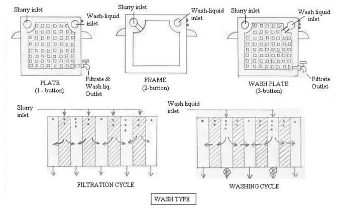
Washing type of plate-frame filter press is required when the cake is to be washed thoroughly with washing liquid (when contaminations are there). Two different types of plates are used. For identification of the plates and frames from outside button systems are there. For example One button: Plate (1)
