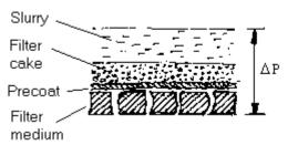
Resistance to filtration is offered by the filter medium, precoat and filter cake.
